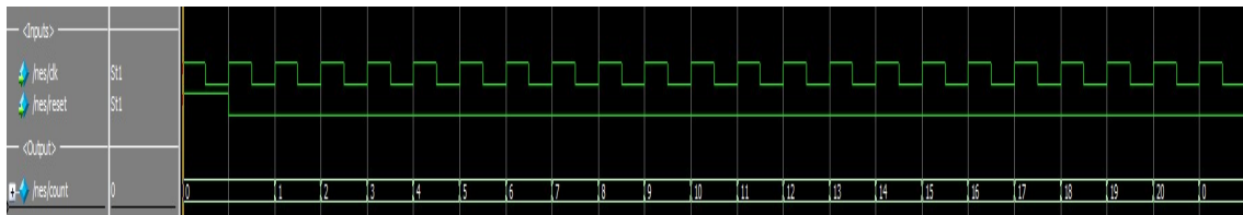
Figure 9: This is the simulation for a simple counter that counts up and is used in timing of the NES reader block.
