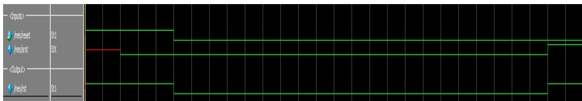
Figure 15: This is the simulation for countreset which is effectively an OR gate used to reset the counter.
