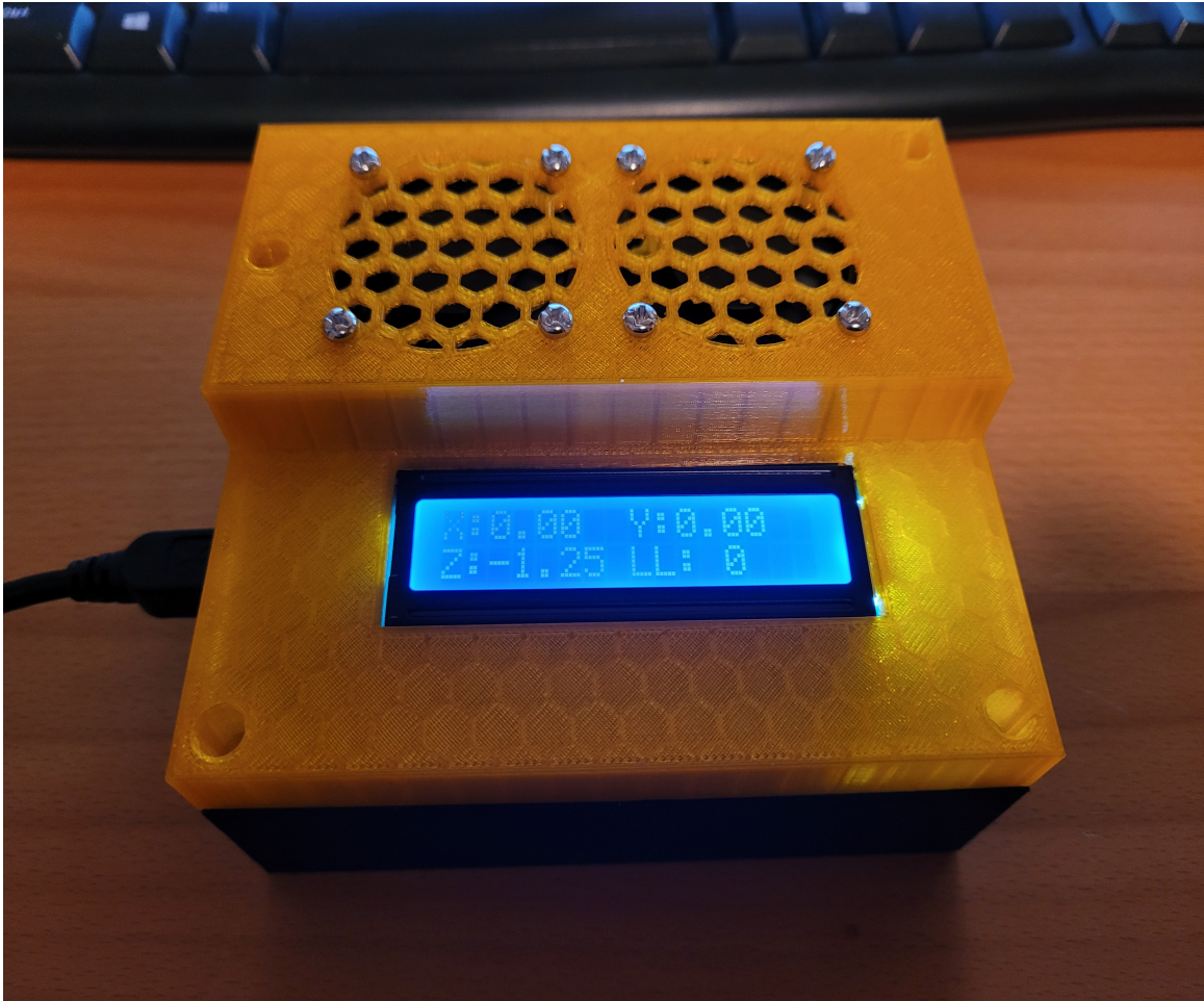
Figure 25: This is an image of the final enclosure with the built PCB inside.
