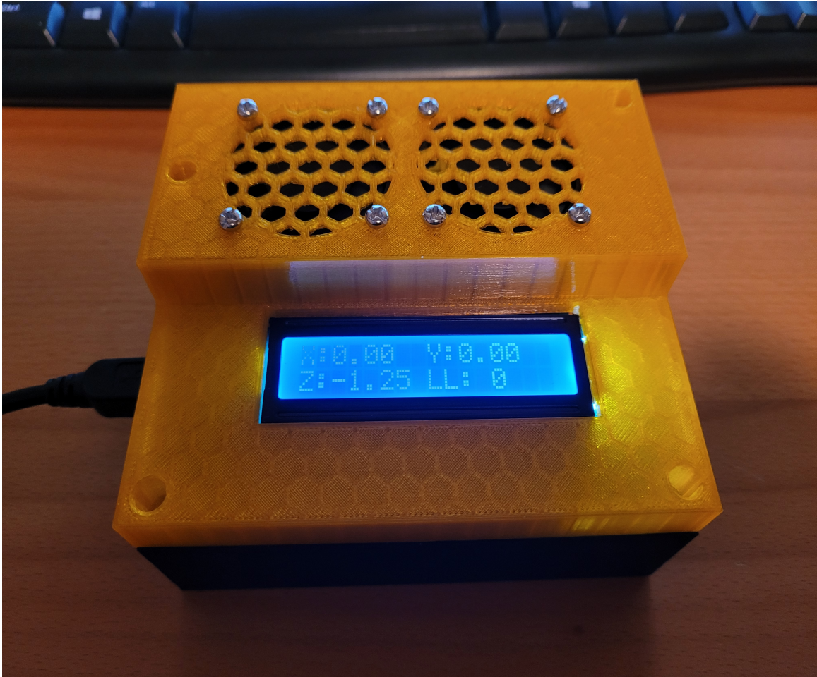
Figure 8: This is a image of what the enclosure looks like with the board and fans inside.
